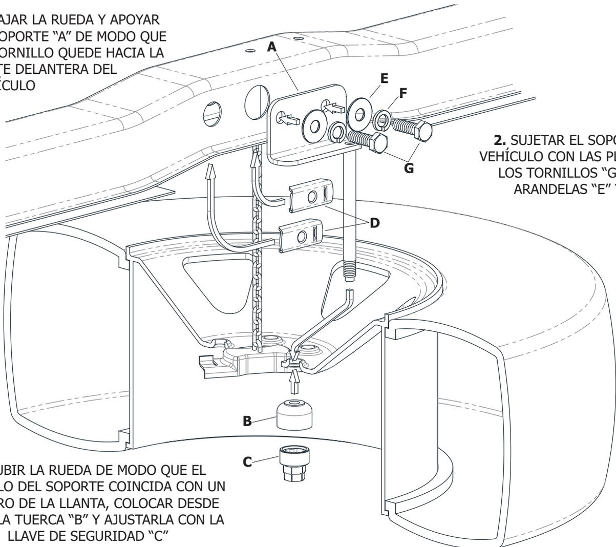
**2.** SUJETAR EL SOPORTE AL VEHÍCULO CON LAS PLACAS "D", LOS TORNILLOS "G" Y LAS ARANDELAS "E" Y "F"
